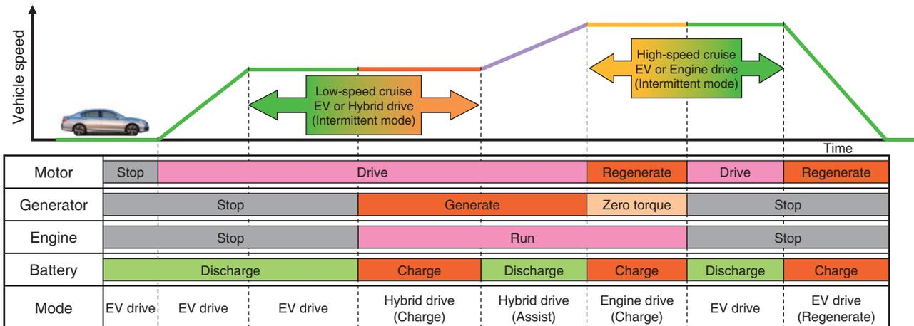
Fig. 7 CS mode operation
