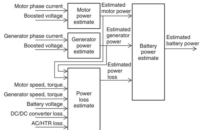
Fig. 13 Battery power estimator
