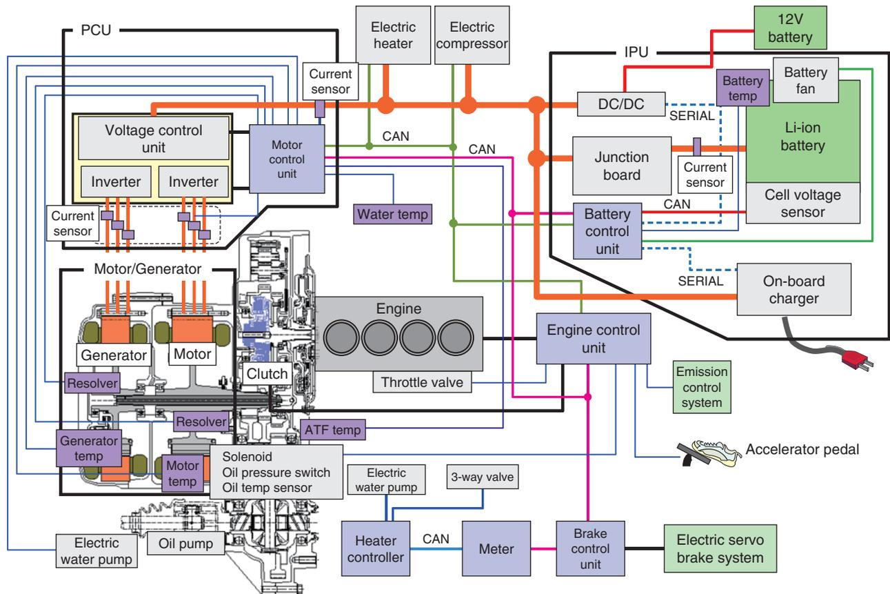
Fig. 5 Block diagram of SPORT HYBRID i-MMD system
