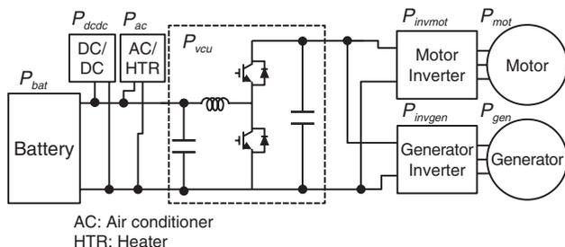
Fig. 12 High-voltage component
